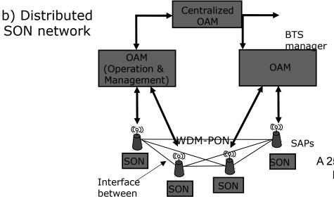
Wave Division Multiplex Passive Optical Network (WDM-PON) to connect Dense Small Cell Networks and SONs of RAN
