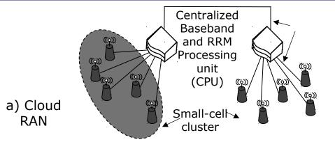
The centralized RAN architecture is one of the most efficient ways to overcome the issues of interference and resource managemens in small cell deployment. However: scalability is lacking.
