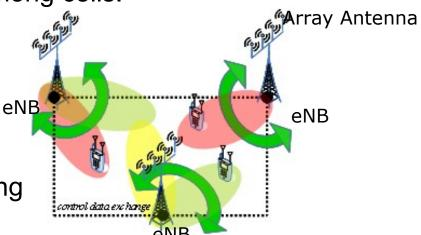
Cooperation of eNBs is based on control information exchanged, rather than real user data exchange.
