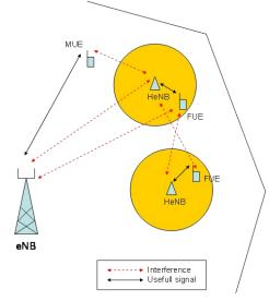
For reducing mutual interference, interference coordination by scheduling of radio resources of the donor (macro) cell to be used by a FC is proposed (reducing capacity of the donor cell).
