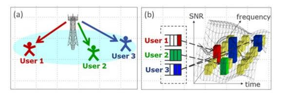
OFDMA multi-user resource allocation: An eNB serving multiple users (a) assigns user data with various QoS requirements (b) to resources in time and frequency taking channel conditions into account. BE traffic is scheduled when possible.
